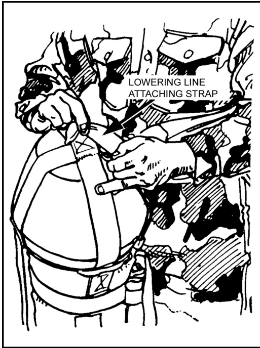
Figure 12-36. Lowering line attaching strap installed.
